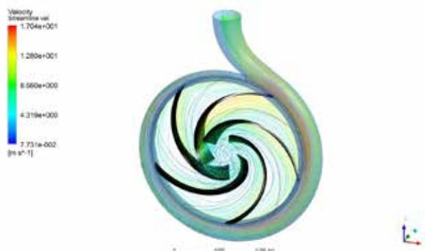
**CFD simulation (Computational Fluid Dynamics) to optimize performance, efficiency and minimize cavitation problems.**
